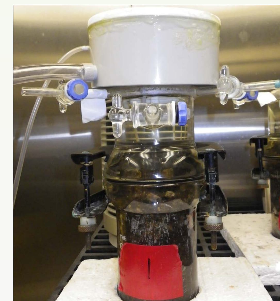
Figure 7: Compressed air from stirrer drives stir bar within mesocosm
